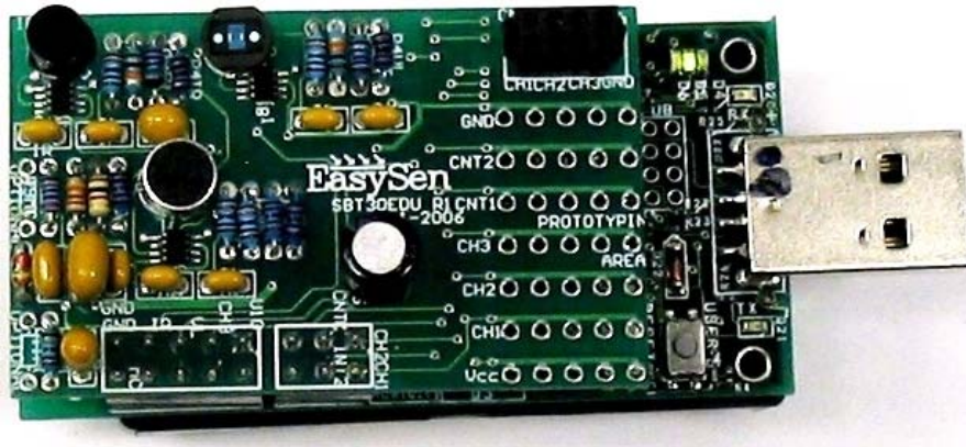
Figure 10. SBT30EDU plugged into a TelosB mote (top view)
